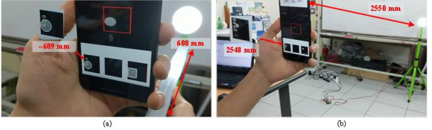
FIGURE 12: Experimental setup for distance measurement: (a) LED light at distance of 600 mm and (b) LED light at distance of 2550 mm from the camera.
